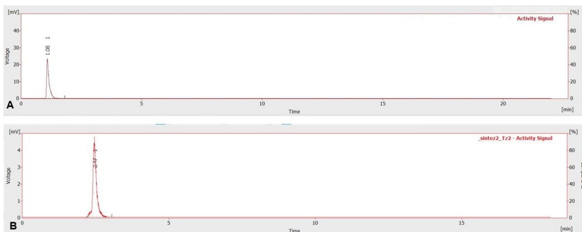
Figure 14 – Radio-HPLC analysis with Tz2 labeling: A – RAD chromatogram of initial [ ^{18}\text{F} ]FDG ( t_r=1.08 min.); B – RAD – chromatogram of labeled product Pr2 ( t_r=2.47 min.)
