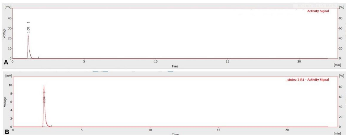
Figure 19 - Radio-HPLC analysis modified R1: A - RAD - chromatogram of initial [ ^{18}\text{F} ]FDG ( t_r=1.08 min.); B - RAD - chromatogram of labeled product Pr3 ( t_r=2.24 min.)
