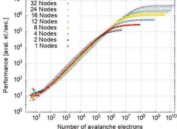
Parallel framework for accounting for space charge effects in simulations of gaseous detectors
